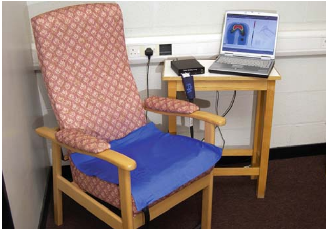
Fig. 7.1 The pressure mapping system.
