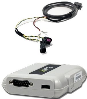
Figure 6: This XRS relay box connects all truck devices (e.g., diagnostics and driver cell) to the XRS fleet management supporting software, which allows data collection.
