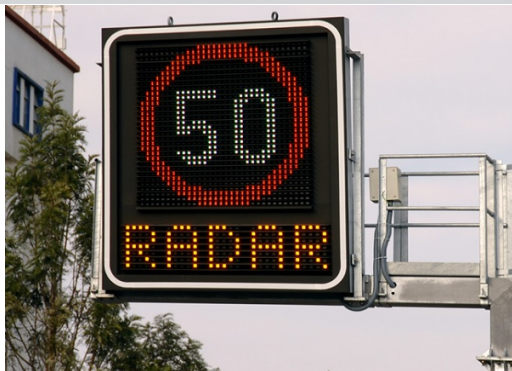
Figure 10: This smart road sign receives data and modifications to better inform drivers and prevent congestion or accidents.
