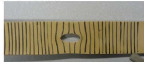
Stress Concentration around Abrupt Change in Cross-Section
