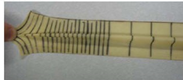
Stress Concentration around Hole
