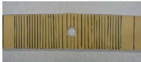
Stress Concentration around Abrupt Change in Cross-Section
