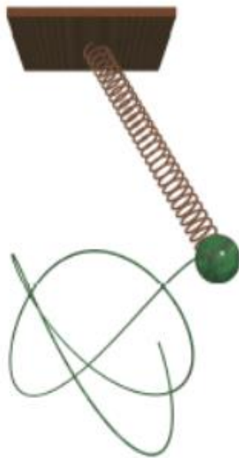
Figure 2.48 A snapshot from a computer program to calculate and animate the motion of a mass–spring system in 3D. This program was written in the language VPython ( http://vpython.org ), which generates real-time 3D visualizations of motion.
