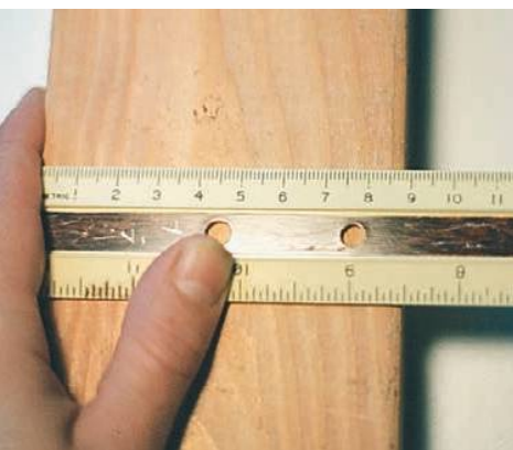
FIGURE 1–5 Measuring the width of a board with a centimeter ruler. Accuracy is about \pm 1 mm.
