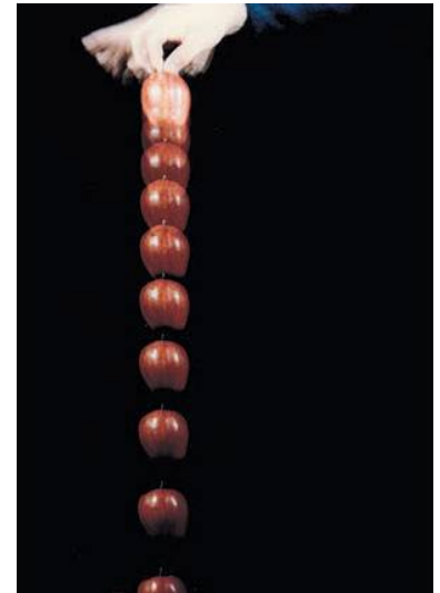
FIGURE 2-19 Multiflash photograph of a falling apple, at equal time intervals. The apple falls farther during each successive interval, which means it is accelerating.
