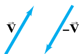
FIGURE 3-7 The negative of a vector is a vector having the same length but opposite direction.
