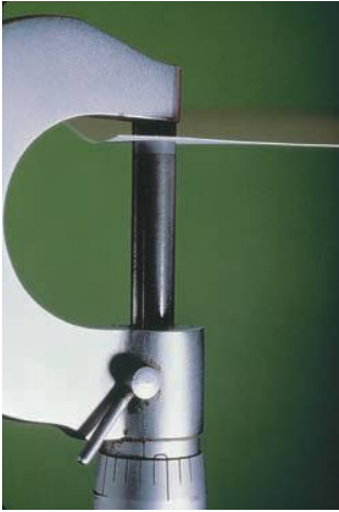
FIGURE 1-11 Example 1-7. Micrometer used for measuring small thicknesses.
