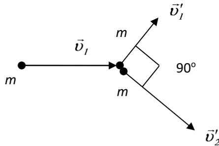
$$\left. \begin{aligned} \vec{p}_1 &= \vec{p}_1' + \vec{p}_2' \quad (\text{τρίγωνο}) \\ \frac{p_1^2}{2m} &= \frac{p_1'^2}{2m} + \frac{p_2'^2}{2m} \end{aligned} \right\} \Rightarrow \left. \begin{aligned} p_1^2 &= p_1'^2 + p_2'^2 + 2\vec{p}_1' \cdot \vec{p}_2' \\ p_1^2 &= p_1'^2 + p_2'^2 \quad (\text{ορθογώνιο}) \end{aligned} \right\} \Rightarrow \vec{p}_1' \cdot \vec{p}_2' = 0 \Rightarrow \vec{p}_1' \perp \vec{p}_2'$$
