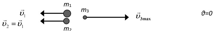
$$p_{3\max} = \sqrt{2Q\mu_{(12)3}} \quad \text{για} \quad \cos \theta = 1 \quad \text{και} \quad v_1 = v_2$$
