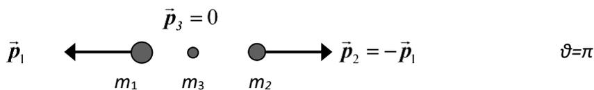
$$p_{3\min} = 0 \quad \text{για} \quad \cos \theta = -1 \quad \text{και} \quad p_1 = p_2 = \sqrt{2Q\mu_{12}}$$
