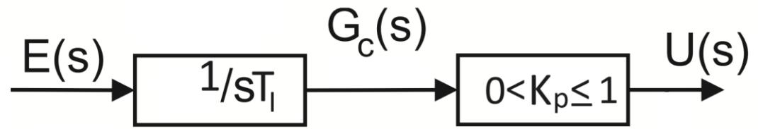
$$\frac{U(s)}{E(s)} = -K_p \frac{1}{sT_I} = -\frac{R_2}{R_1 + R_2} \frac{1}{sRC} \Rightarrow K_p = \frac{R_2}{R_1 + R_2}$$
