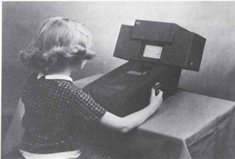
FIG. 1. A recent model of a teaching machine for the lower grades. The machine operates on the principles described in the accompanying article. Material is presented in a window with a few letters or figures missing. The pupil moves sliders which cause letters or figures to appear. When an answer has been composed, the pupil turns a crank. If the answer was right, a new frame of material moves into the window and the sliders return to their home position. If the answer was wrong, the sliders return but the frame remains and must be completed again. (This is a later version of the device described in Skinner's 1954 paper.)
