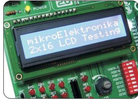
Figure 28 LCD 2x16 in 4-bit mode
