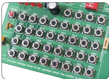
**Figure 23** Pushbuttons
