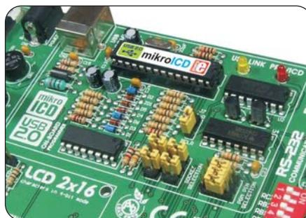
**Figure 17** On-Board USB programmer with mikroICD
