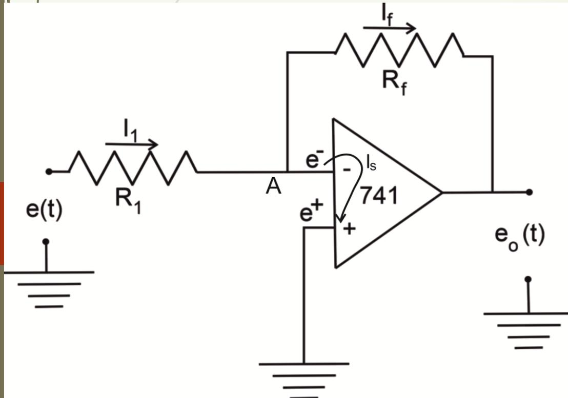
$$I_1 = I_s + I_f \xrightarrow{I_s=0} \frac{e(t) - e^-}{R_1} = \frac{e^- - e_o(t)}{R_f}$$
