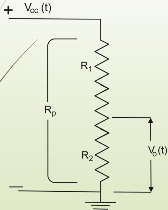
$$V_o(t) = \frac{R_2}{R_1 + R_2} V_{cc}(t)$$
