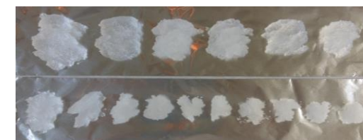
Volume reduction of SAP due to salt concentration increase
